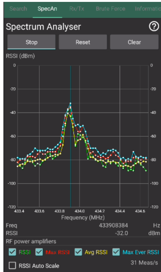
Figure 32. The frequency analyzer of the PandwaRF tool showing our remote's signal
