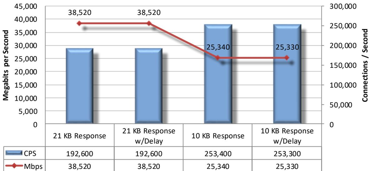
Figure 10 – HTTP Capacity with Transaction Delays
