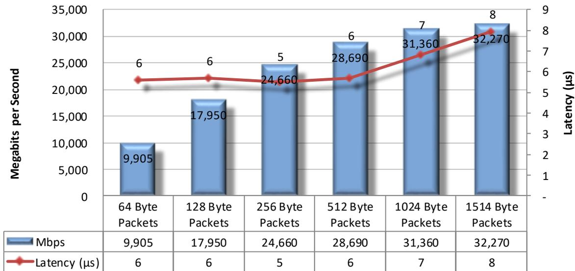
Figure 13 – Raw Packet Processing Performance (UDP Traffic)
