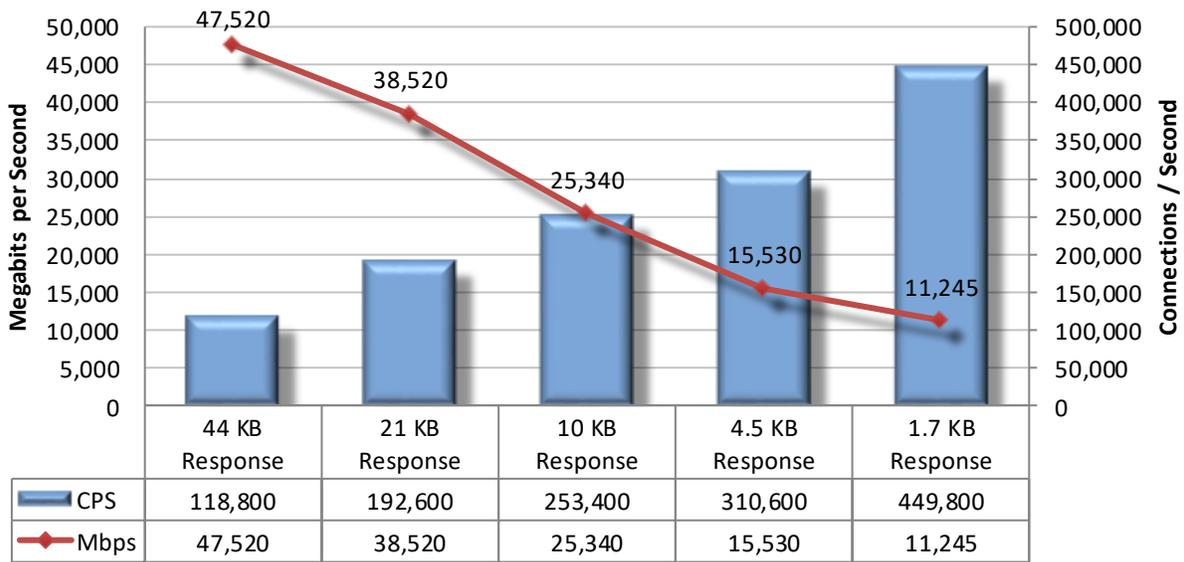
Figure 9 – HTTP Connections per Second and Capacity
