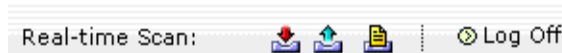
FIGURE 3-8. Title bar showing Real-time Scan with incoming, outgoing, and running file scanning enabled
