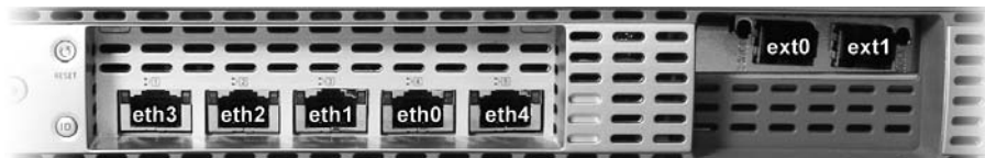
FIGURE 5-3. NVW 2500 system names for seven ports
