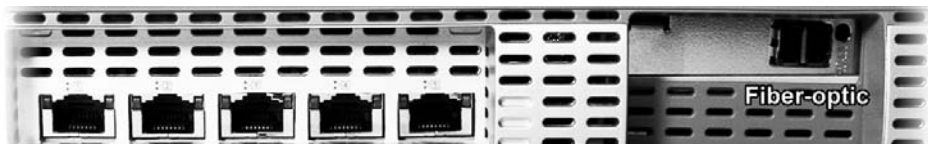
FIGURE 1-3. Network VirusWall 2500 Ethernet ports 1 through 6 with five copper ports and one multi-mode fiber-optic port
