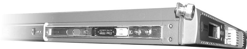
FIGURE 2-13. Completed rack ear and rail preparation
