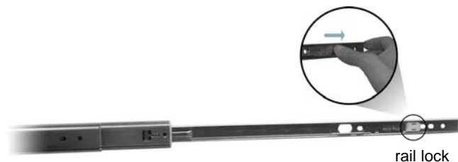
FIGURE 2-10. Detaching the rail from the slide
