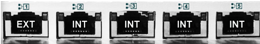
FIGURE 3-12. Interface allocation for a port grouping deployment
