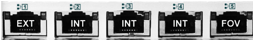
FIGURE 3-15. Interface allocation for a port grouping with failover deployment
