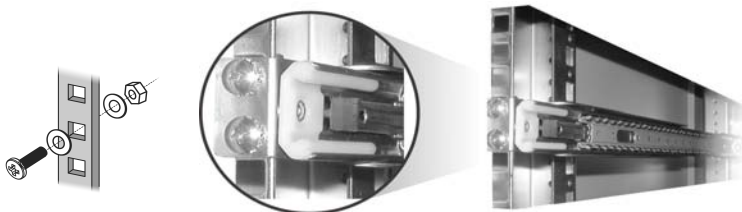
FIGURE 2-23. Installing the cage screws in the top and bottom holes of the slide set (front vertical rail view)
