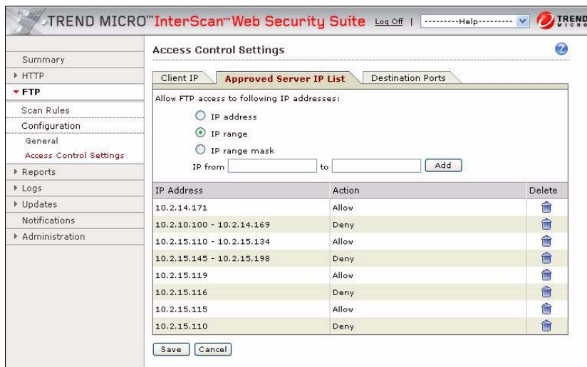
FIGURE 8-4 Access Control Settings Approved Server IP List tab
