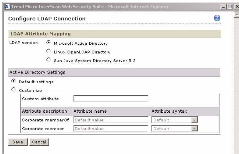
FIGURE 4-3 Choose your directory (LDAP) server's vendor in the Configure LDAP Connection screen
