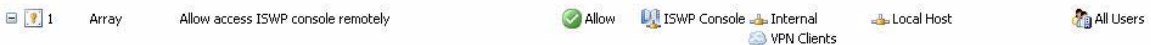
FIGURE 2-20 Allow access to the local host from internal network and VPN client.
