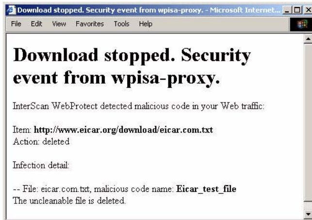
FIGURE 3-9. This warning screen shows the detection of an EICAR test virus.
