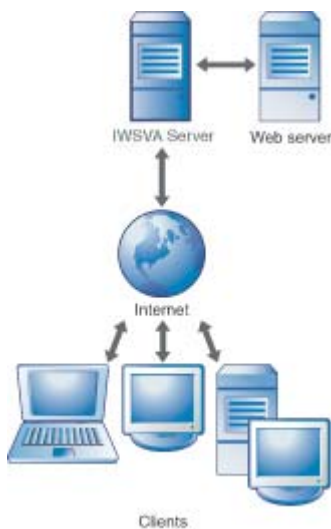
FIGURE 2-15 Reverse proxy protects Web server from clients
