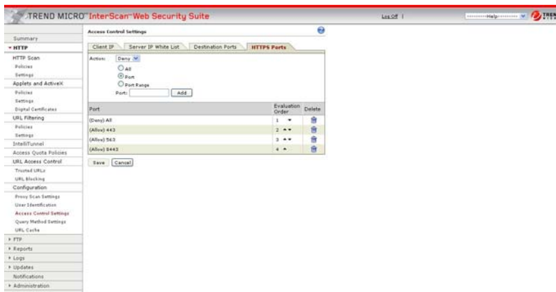
FIGURE 5-2 Allow access to the secure port (typically 8443) if using DCS and the HTTPS management console
