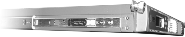
FIGURE 103. Completed rack ear and rail preparation
