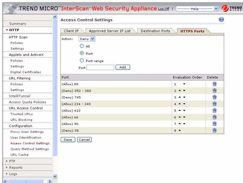
FIGURE 13. HTTPS port access can be selectively allowed or denied on the HTTPS Ports tab
