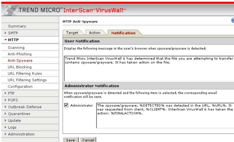
FIGURE 4-4. HTTP Anti-Spyware screen, Notification tab with default message text and with Administrator check box selected
