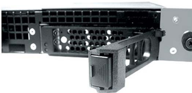
FIGURE D-4. Hard disk release lever
