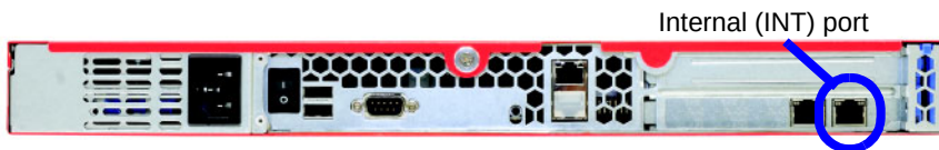
FIGURE 15-10. The appliance back panel showing location of internal (INT) port
