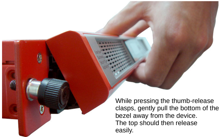
FIGURE D-2. Releasing the bezel
