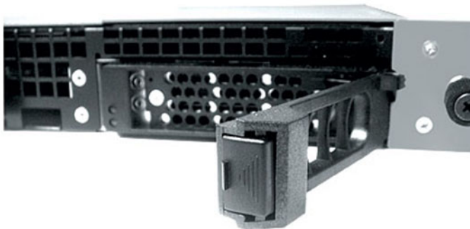
FIGURE D-4. Hard disk release lever
