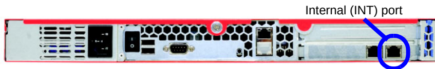
FIGURE 14-10. The appliance back panel showing location of internal (INT) port
